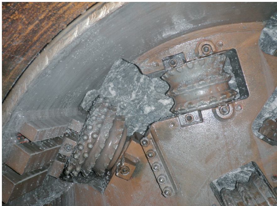
Roller cutter can be replaced from inside chamber.
