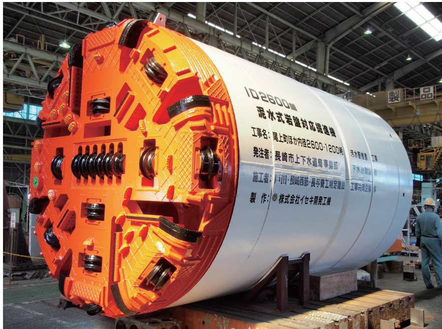
Cutter head structure is applied to "intermediate support".
